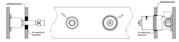
7. Waterproof the gap between the plasterboard and body.
