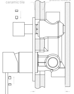
1. Fix body on noggin and ensure installation depth is 62-76mm from noggin to ceramic tile.
