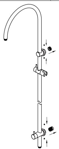
6.Locate and put shower rail assembly onto wall adaptors. Tighten grub screws firmly with allen key provided.
