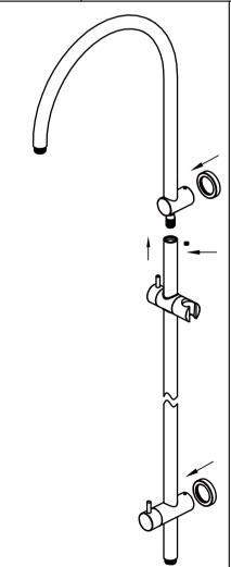
5.Screw shower rail into shower arm component. Tighten firmly. Push 2 back plates onto shower arm component and body
