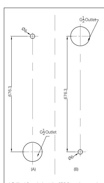
1.Drill a  $\varphi 6mm$  hole at the 676.3mm downwards or upwards outlet vertical downward or upward position, as the picture A and B.
