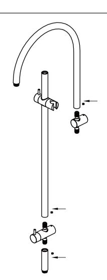
4.Unscrew 3grub screws as picture and unplug short shower rail, long short rail and shower arm one by one. Change the place of body and bracket. Then plug in short shower rail, long shower rail and shower arm and screw the 3 grub screws.
