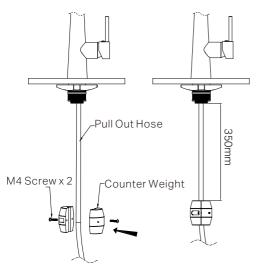
5. Install counter weight by tightening the screws, please note that the distance from counter weight to bottom of thread connector is 350mm, as shown in figure.
