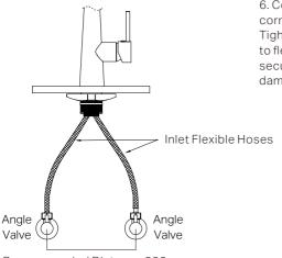
6. Connect the inlet flexible hoses to the corresponding hot and cold water supply valves. Tighten the female cone nuts by hand (according to flexible hose instruction), ensuring they are secure yet not overtightened to avoid thread damage.
