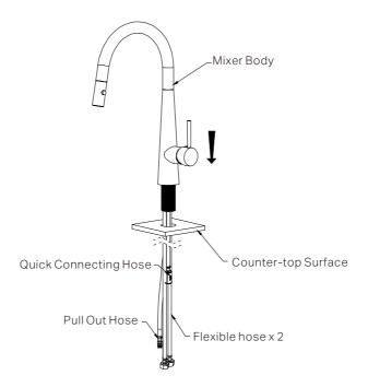
2. Place the mixer body and pass the flexible hoses, pull out hose and quick connecting hose through the hole in the counter-top.
