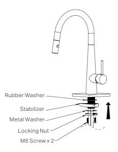
3. Install the rubber and metal washers, if a stabilizer is required, install the stabilizer after positioning the rubber washer.
