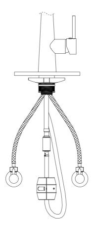
7. Check all connections for leaks. If any fittings are leaking, shut off the water as necessary to stop the leaks.
