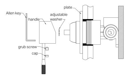
6.Slide the backplate onto the wall.7. Attach the washer to the cartridge rod, position the handle, tighten it with a grub screw using an Allen key, and cap the grub screw hole.
