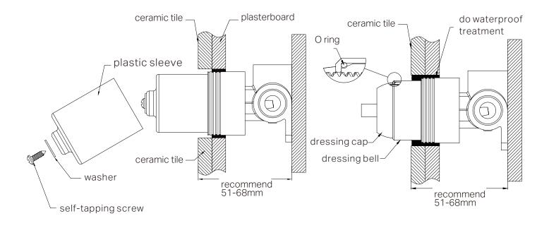
$1.Drill \, a \, \phi 50 mm$  hole in the ceramic tile, then  $\ position$  it as shown in the above diagram.
