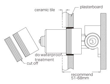
Secure the mixer body (1) to the nogging, ensuring an installation depth of 51-68mm from the nogging to the ceramic tile. Note: Do not remove the plastic sleeve (2) from the mixer body.
