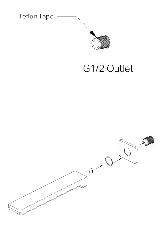
Installing the backplate:
