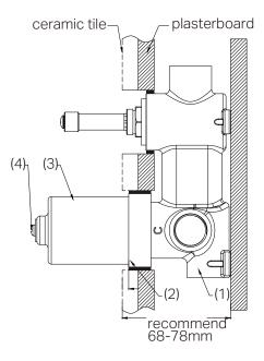
4. When the installation depth is 68-70mm, make the plastic sleeve (2) 2-4mm from ceramic tile surface to body.
