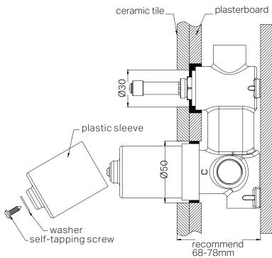
1.Drill a  $\phi 50mm$  and a  $\phi 30mm$  hole in the ceramic tile, then position it as shown in the above diagram.
