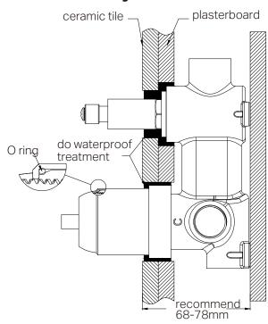
3. Insert the O ring to the dressing bell groove, and slide the cartridge bell onto cartridge and slide divertor dressing bell onto divertor cartridge.
