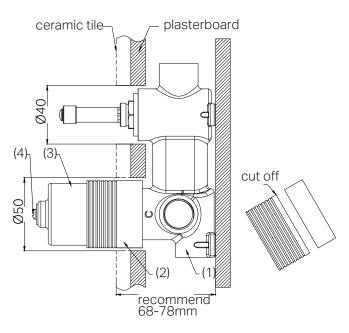
1. Secure the mixer body (1) to the nogging, ensuring an installation depth is 68-78mm from the nogging to ceramic tile.
