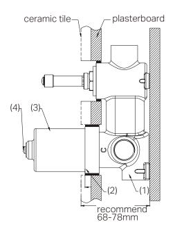
4. When the installation depth is 68-70 mm, make the plastic sleeve (2) 2-4 mm from ceramic tile surface to body.
