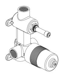
7. Waterproof for the gap the plasterboard and body.
