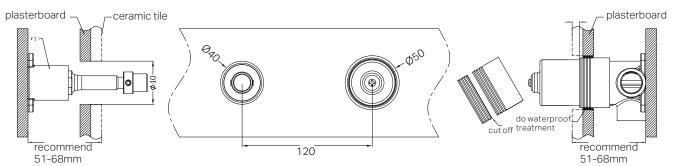
4. Mark the plastic sleeve (2) 4-7mm from the ceramic tile surface to the body and waterproof the gap between the plasterboard and body.
