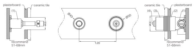
1. Secure the mixer body (1) to the nogging, ensuring an installation depth of 51-68mm from the nogging to the ceramic tile. Note: Do not remove the plastic sleeve (2) from the mixer body.
