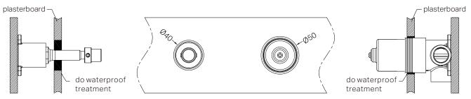
7.Waterproof the gap between the plasterboard and body
