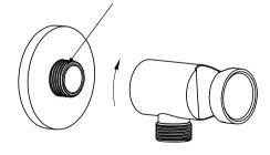
3. Pull back plate onto the outlet, and screw shower bracket body onto outlet.
