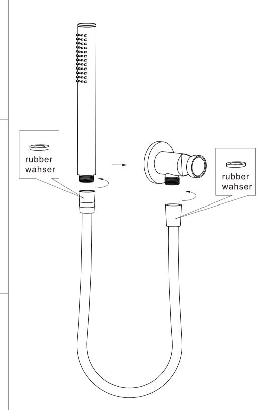
4. Connect bracket and hand shower with hose. TEST & CHECK FOR LEAKS.
