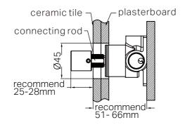
3. Adjust connecting rod and ensure depth is 25-28mm from the front of adaptor to ceramic tile. Drill a  $\phi$  45 hole on plasterboard and ceramic tile for the body, according to above picture. Then install plasterboard and do waterproof for the whole plasterboard. Install ceramic tile.
