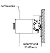
1. Fix body on nogging and ensure installation depth is 51-66mm from nogging to ceramic tile. ceramic tile
