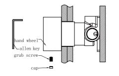
3. Make hand wheel into connecting rod, turn the hand wheel counterclockwise to the end. Then reinstall the hand wheel, make the "C" should be on twelve o'clock direction and "H" on the six o'clock direction, according to above picture. Then tighten grub screw of hand wheel by allen key, put cap into hand wheel.
