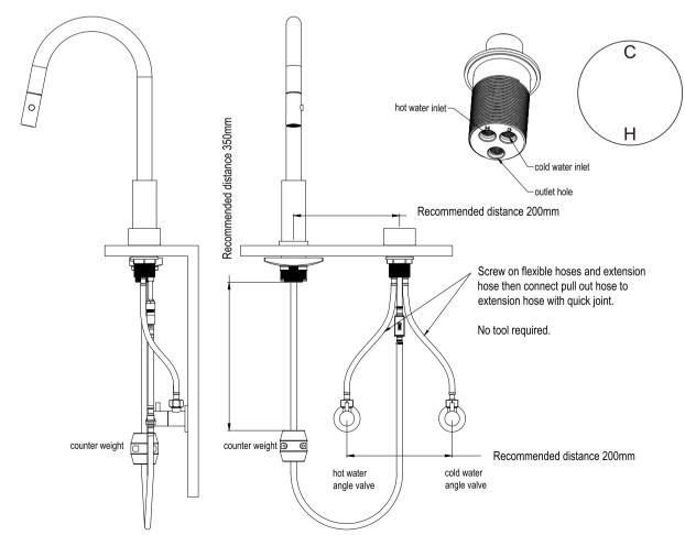
7. Turn the hand wheel counterclockwise to the end. Then reinstall the hand wheel, make the "C" should be on twelve o'clock direction and "H" on the six o'clock direction, according to above picture. Then tighten grub screw of hand wheel by allen key, put cap into hand wheel.
