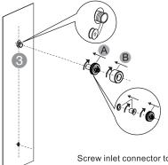
Screw inlet connector to the water supply pipe.
