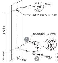
Drill hole according to the dimension. Anchor into the wall. then secure the base plate to the wall by usingscrew.
