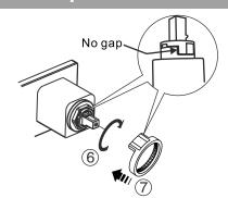
\* Move the pivot of cartridge to the position of you wanted hot water temperature. Reinstall the temperature limiter with no gap as shown in the figure above.
