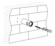
5. Position the rod bracket hole to the left and secure the bracket with expansion screws, as shown in the image.
