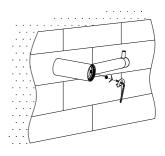
4. Remove the rod of the toilet roll holder by unscrewing the grub screw.
