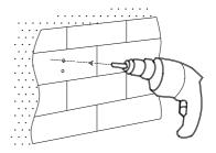
2. Use an electric drill with a 6mm drill bit to drill holes at the marked points.
