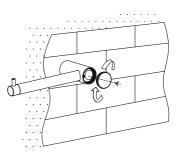
6. Install the rod of the toilet roll holder by tightening the grub screw, and screw on the cap.
