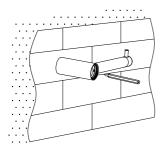
1. Unscrew the cover from the toilet roll holder. Place the toilet paper holder in the desired installation position as shown. Mark the center of the mounting bracket through the support with a marking pen.
