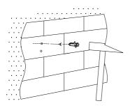
3. Insert the expansion plugs into the drilled holes using a hammer.
