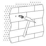
3. Insert the expansion plugs into the drilled holes using a hammer.
