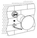
5. Install the robe hook onto the fixing bracket and secure it by tightening the grub screw.
