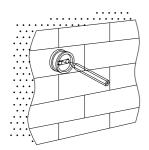
1. Use the fixing bracket to mark the drilling points on the wall.
