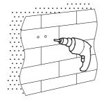
2. Use an electric drill with a 6mm drill bit to drill holes at the marked points.
