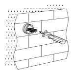
4. Place the fixing bracket covers over the holes and secure them firmly with expansion screws.
