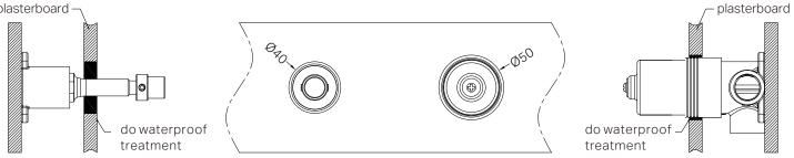
7.Waterproof the gap between the plasterboard and body
