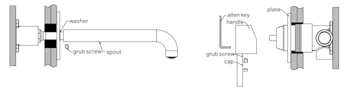
6. slide the backplate and washer onto the wall, set the spout in place, and secure it tightly using the grub screw.
