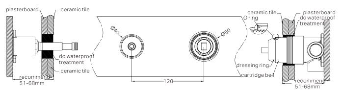
3. insert the oring to the cartridge bell groove, and slide the dressing ring onto cartridge.
