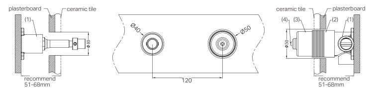
1. Secure the mixer body (1) to the nogging, ensuring an installation depth of 51-68mm from the nogging to the ceramic tile.
