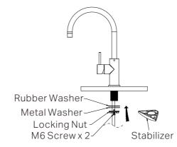
3. Install the rubber and metal washers, if a stabilizer is required, install the stabilizer after positioning the rubber washer. Tighten the locking nut securely with the two M6 screws to ensure the mixer is firmly attached to the counter-top. Avoid over tightening to prevent damage to the components.
