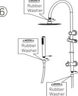
Screw the overhead shower into the shower arm, ensuring a rubber washer is in place for watertight seal.
