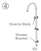
Positioning the divertor and shower bracket as in Figure D.
