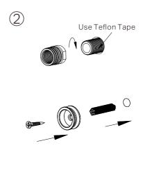
Ensure the G1/2 outlet thread is the correct length, cut to the outlet if required.
