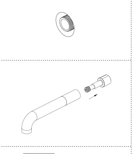
1. Cut off the G1/2 outlet thread to flush with the finished wall surface.
