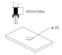
1. Pre-drill or create a hole with a diameter of 35mm at the proper location. Please note that the thickness of the surface should be between 3mm-40mm.
