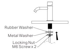
3. Install the rubber and metal washers, tighten the locking nut securely with the two M6 screws to ensure the mixer is firmly attached to the counter-top.
