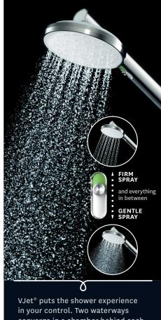
VJet® puts the shower experience in your control. Two waterways converge in a chamber behind each nozzle to create a spinning vortex that seamlessly changes speed as you adjust the slider. Resulting in a smooth transition from a firm invigorating spray, to a gentle spray, and everything in between uniquely tailored by you.
