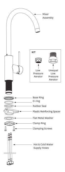
**Important:** Before you begin, turn off the water supply. It is recommended to fit isolation valves to both the hot and cold supply.
