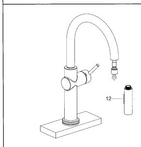
Ensure all connections are tightened and the handle is in the off position.
