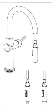
Turn on the handle gently. Turn clockwise for cold water, counter-clockwise for hot water.
